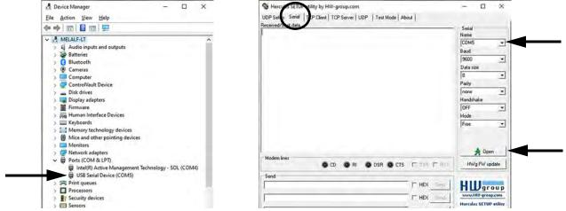
Figure 4-2. Connecting to a Serial Port
