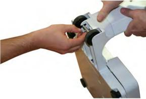
Figure 2-4. Attach Wheel Assembly
