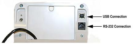
Figure 4-1. Connection Ports
