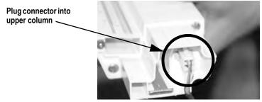
Figure 2-5. Extend Cable Through Scale Column
