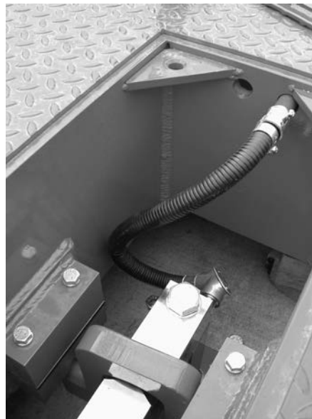
Figure 4-4. Load cell Access
