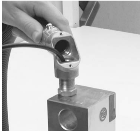
Figure 4-3. Installing 90° Fitting to Load Cell
