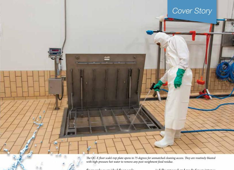
floor scale as an ideal floor scale choice to LALA. The QC-X floor scale's 304 stainless steel frame is
