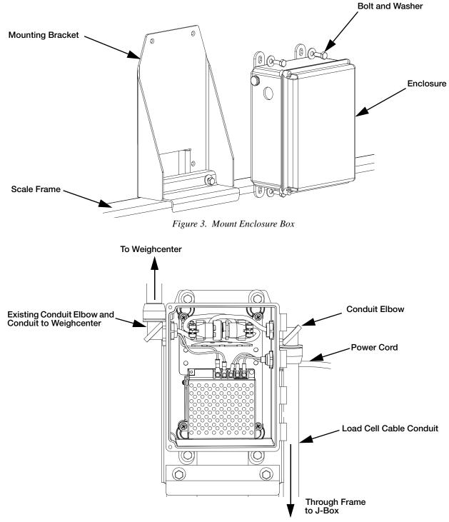
Figure 4. Wiring Diagram
