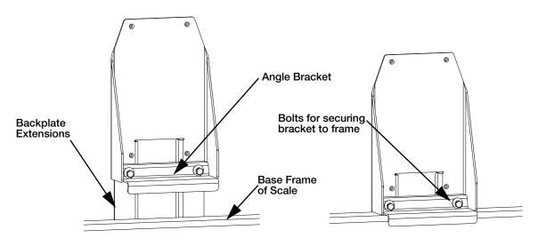
Figure 2. Mounting Power Box Assembly to Frame
