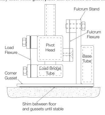
Figure 2-1. Side View - Pivot Head
