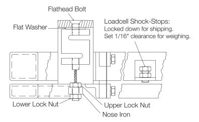
Figure 4-1. Load Cell Mounting
