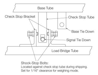
Figure 2-2. Top View - Check Stops and Tie Downs
