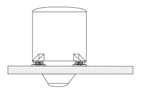
Figure 2-1 Preferred Weigh Module Orientation
