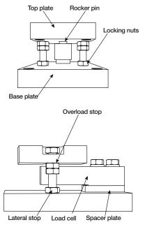
Figure 2-3 Lateral and Overlift/Overload Stops
