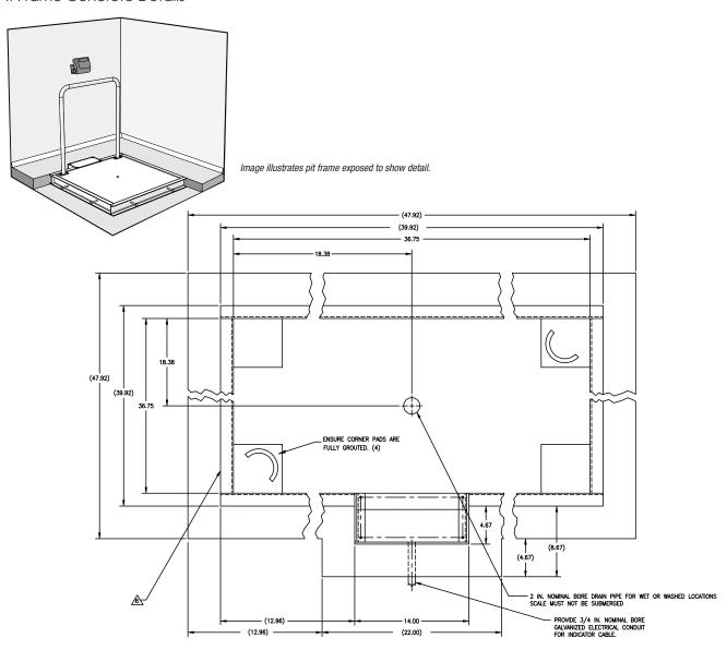
NOTE: HANDRAIL ON SCALE WILL MOUNT ON SAME SIDE AS JUNCTION BOX POCKET
