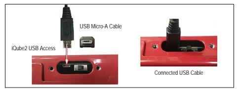
Figure 1. Firmware Update Cable Connection
