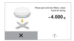
▶ Place an empty sample pan on the analyzer, along with one or two filters if necessary.
