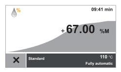
If no target value is set, the measurement process is displayed as a curve diagram.
