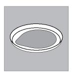
Affix the pad to the center of the sample pan, sticky side down.
