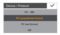
➤ To open the PC spreadsheet format menu item on the moisture analyzer, go to USB port and select Device/Protocol.
