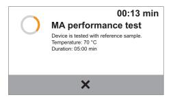
➤ The display shows the progress of the test and the remaining time.
