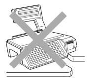
•Always operate the scale on a level surface.
