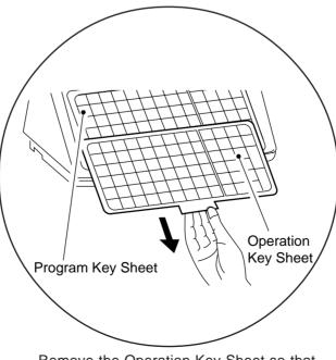
Remove the Operation Key Sheet so that the Program Key Sheet under it can be used.
