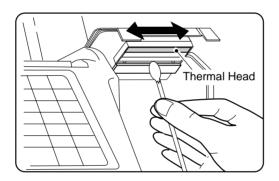
Dip the end of the cotton swab into cleaning fluid and wipe the thermal head.
