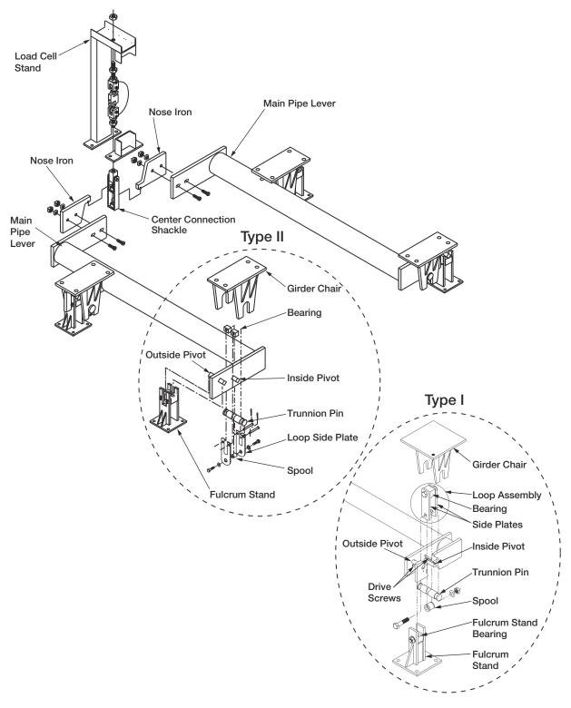
Figure 2-1. Pipe Lever Assembly
