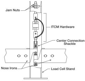
Figure 2-2. Load Cell Assembly
