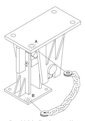
Figure 3-1. Safety Chain Option Assembly
