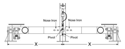
Figure 2-4. Nose Iron Adjustment
