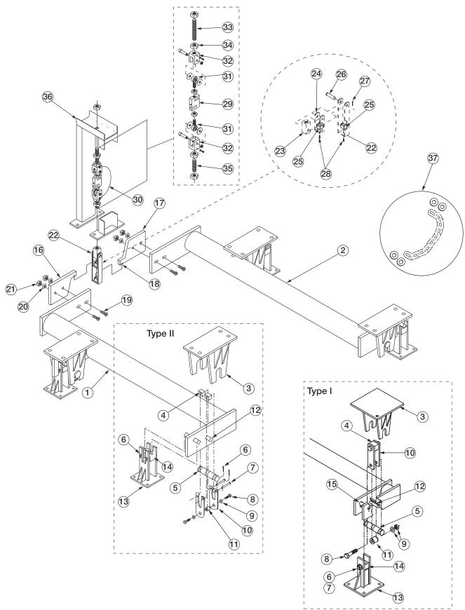
Figure 4-1. Pipe Lever Scale Parts Illustration
