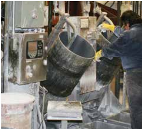
Rubber granules are first mixed with a special blend of adhesives, and then portioned into a heated press to be formed into flooring tiles.
