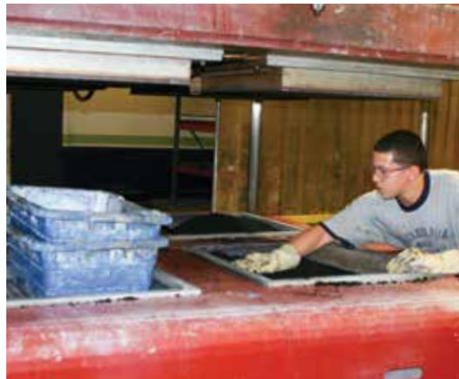
Rubber granules are first mixed with a special blend of adhesives, and then portioned into a heated press to be formed into flooring tiles.
