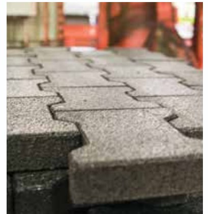
Rubber granules are first mixed with a special blend of adhesives, and then portioned into a heated press to be formed into flooring tiles.
