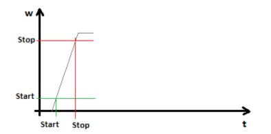
• Unload step (Trigger 3 from release 1.01.00): points started to be sent when the weight is less of equal to on value and stopped to be sent when the weight is less or equal to off value
