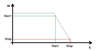
• Unload pulse (Trigger 4 from release 1.01.00): points started to be sent when the weight is less of equal to on value and stopped to be sent when the weight is greater or equal to off value
