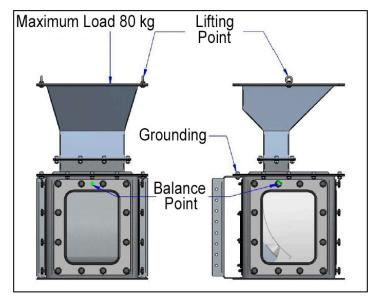
Figure 2-1. Lifting Points
