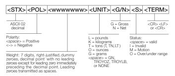
Figure 12-1. Continuous Output Serial Data Format
