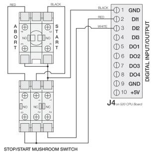
Figure 11-7. Batching Switch Wiring Diagram
