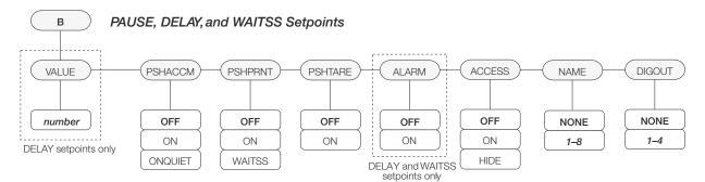
Figure 11-3. Submenu for PAUSE, DELAY, and WAITSS Setpoints
