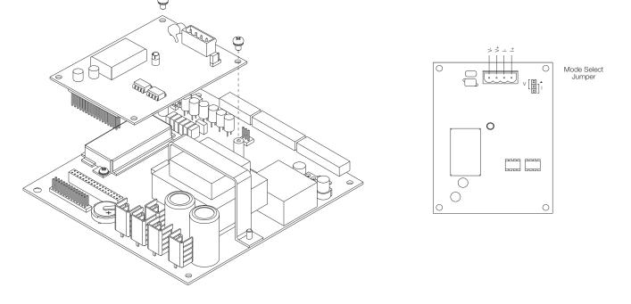
Figure 2-7. Analog Output Card Installation
