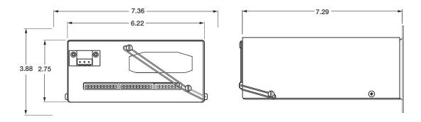
Figure 2-3. 520 Stainless Steel Panel Mount Dimensions
