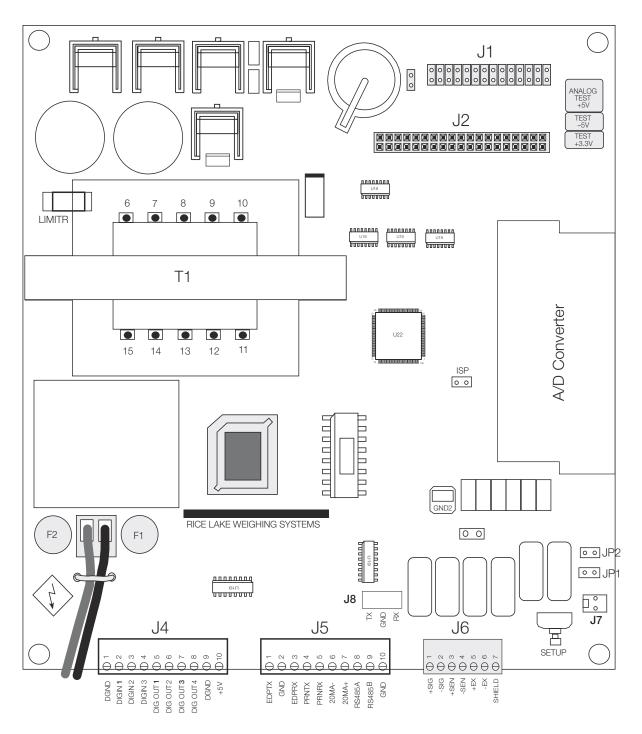
Figure 2-6. 520 CPU and Power Supply Board
