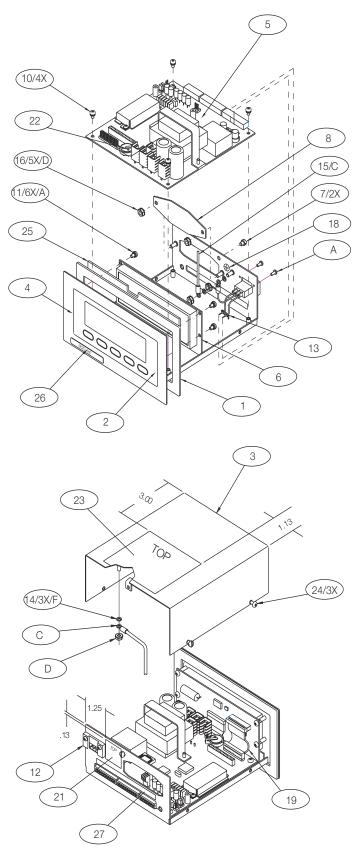
Figure 2-9. Stainless Steel Panel Mount Model Assembly
