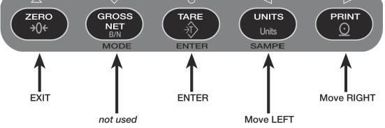
Figure 12-6. Front Panel Key Functions in Test Mode
