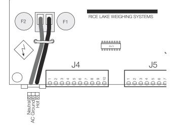
Figure 2-5. AC Power Cord Connection Location
