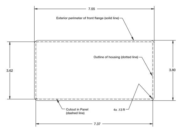
Figure 2-2. 520 Desktop Model Panel Mount Cut Out
