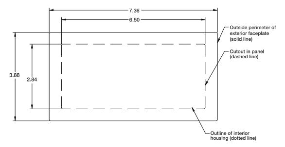
Figure 2-1. 520 Stainless Steel Panel Mount Cut Out
