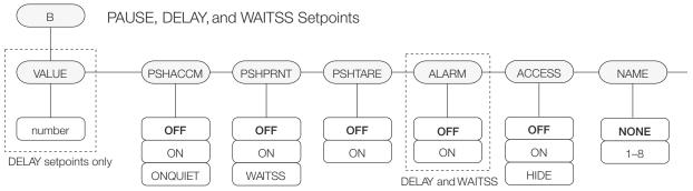
Figure 3-13. Submenu for PAUSE, DELAY, and WAITSS Setpoints
