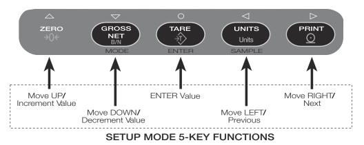
Figure 3-2. Five-Key Keypad Functions in Setup Mode
