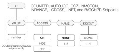
Figure 3-14. Submenu for COUNTER, AUTOJOG, COZ, INMOTON, INRANGE, -GROSS, -NET, and BATCHPR Setpoints
