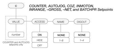
Figure 11-4. Submenu for COUNTER, AUTOJOG, COZ, INMOTON, INRANGE, -GROSS, -NET, and BATCHPR Setpoints
