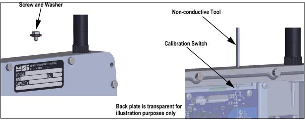
Figure 5-1. Press Configuration Switch
