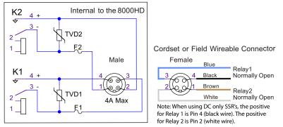
Figure 6-5. Cordset or Field Wireable Connector
