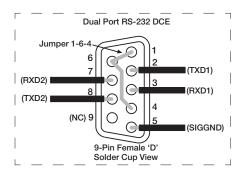
Figure 6-2. Communications Port 1 Wiring
