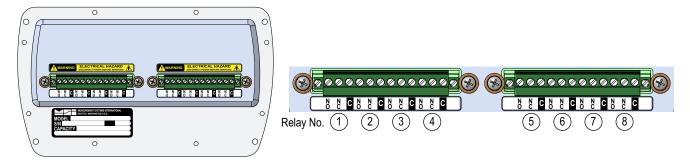
Figure 6-6. Extended Relay Kit:
