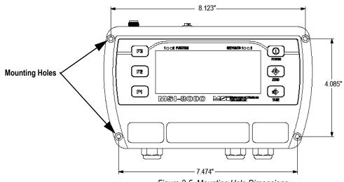
Figure 2-5. Mounting Hole Dimensions
