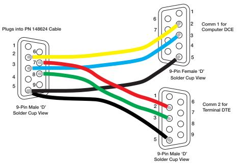
Figure 6-4. Connection with Y Adapter
