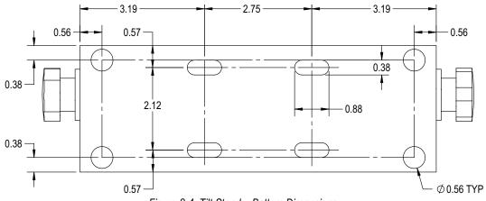
Figure 2-4. Tilt Stand – Bottom Dimensions
