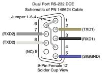
Figure 6-1. Standard Adapter Cable (PN 148624)
