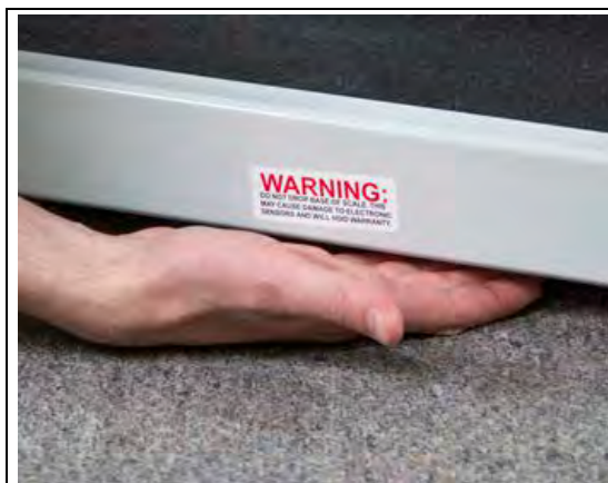
Figure 2-5. Scale Base Clearance
