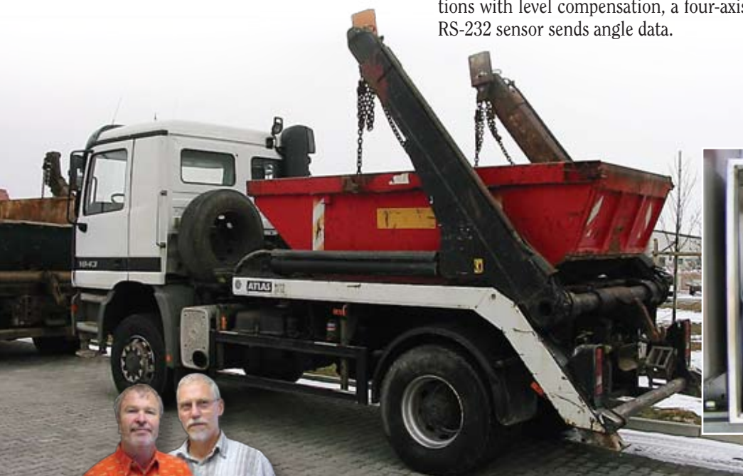
Heinz and Horst's goal was to develop a more accurate on-board weighing system approved as Class III, with a maximum number of verification intervals up to 3,000.
