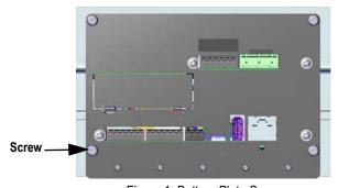
Figure 1. Bottom Plate Screw
