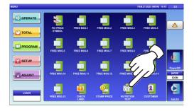
2-1, The "Nutrition Text" screen is displayed. To create the first text, press the [NEW] button.
