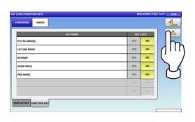
**3.** Press the "PASSWORD" field to display the keypad. Then, enter a 6-digit password and press the [SET] key on the keypad.
