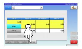
**3.** Press the input field at the right-bottom of the screen to display the keypad. Then, enter a PLU number and press the [PLU] key on the keypad.
