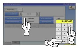
6. To enter the start time, press the "START TIME" field, enter a numerical value, and press the [SET] key on the keypad.
