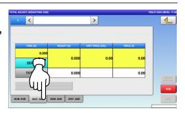
**3.** Press the input field at the right-bottom of the screen to display the keypad. Then, enter a PLU number and press the [PLU] key on the keypad.
