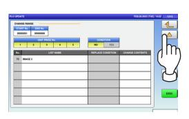
2. Enter the start and end numbers and press these fileds respectively to specify the target PLUs.
