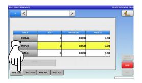
**3.** Press the input field at the right-bottom of the screen to display the keypad. Then, enter a PLU number and press the [PLU] key on the keypad.
