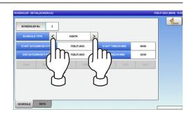
**5.** To enter the start date, press the "START DATE" field, enter a numerical value, and press the [SET] key on the keypad.
