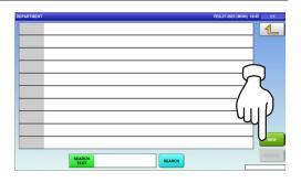
2-2. To call up desired data, press the Input field at the bottom right of the screen to display the keypad. Then, enter a numerical value and press the [PLU] key on the keypad.
