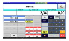
**14.** Enter the weight, and press the "Fixed Weight" field on the screen.
