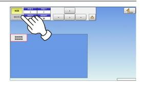
6. Set desired key size and position by using the input fields and arrow buttons, followed by pressing the [SET] key on the keypad.
