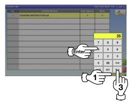
**2-3.** To change existing data, press a desired field for selection and then the [DETAIL] button.
