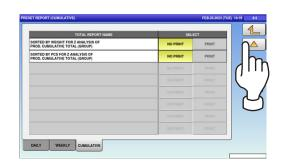
**4.** Select a desired report type by pressing the corresponding tab, and press any selection buttons to set whether or not to print the total.
