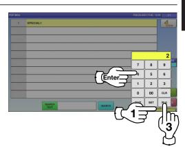
**2-3.** To change existing data, press a desired field for selection and then the [DETAIL] button.
