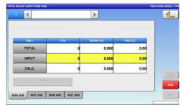
2. To display the "Total Adjust (Weighing Add)" screen, press the [WGT. ADD] tab.
