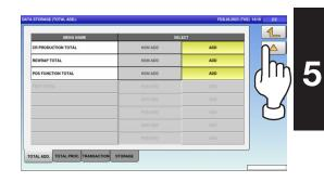
2. Press any selection buttons to set whether or not to apply the total addition function for each menu.
