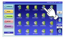
2. The Preset Key screen is displayed. Press a desired field for selection, and press the [DETAIL] button.
