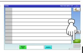
**2-2.** To call up desired data, press the Input field at the bottom right of the screen to display the keypad. Then, enter a numerical value and press the [PLU] key on the keypad.
