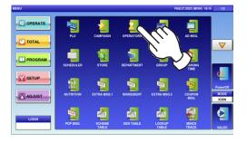
2. The "Operator" screen is displayed. To call up desired data, press the Input field at the bottom right of the screen to display the keypad. Then, enter a numerical value and press the [PLU] key on the keypad.
