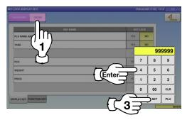
**4** Select a desired key category by pressing the corresponding tab, and press any selection buttons to lock or unlock lock the key.
