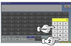
**3.** Press the [COPY] key while the number is displayed in the INPUT field.
