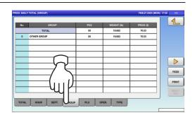
**5.** Press the input field at the right-bottom of the screen to display the keypad. Then, enter a desired PLU number and press the [PLU] key on the keypad.
