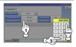
**8.** To enter the end time, press the "END TIME" field, enter a numerical value, and press the [SET] key on the keypad.
