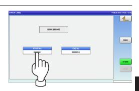
**3.** Enter the start number and the end number via the keypad, and press the [SET] key.
