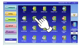
$2_{-1}$  The "Store" screen is displayed. To call up desired data, press the Input field at the bottom right of the screen to display the keypad. Then, enter a numerical value and press the [PLU] key on the keypad.
