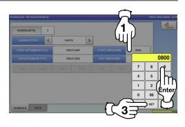
7. To enter the end date, press the "END DATE" field, enter a numerical value, and press the [SET] key on the keypad.
