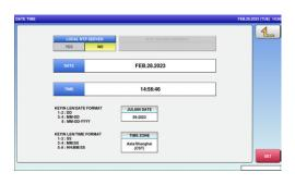
2. To change the date, press the "DATE" field and enter a new date data. Then, press the [SET] key.
