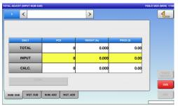
2. To display the "Total Adjust (Input Number Addition)" screen, press the "NUM. ADD" tab.
