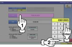
**3.** To change the time, press the "TIME" field and enter a new time data. Then, press the [SET] key.
