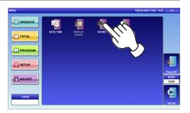
2. The "Sound" screen is displayed. To set sound levels, press "ON" in the "Sound" field and press [<] or [>].
