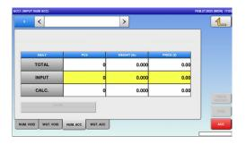
2. Press the "WGT. ACC" tab to display the "Weighing Accumulation" screen.
