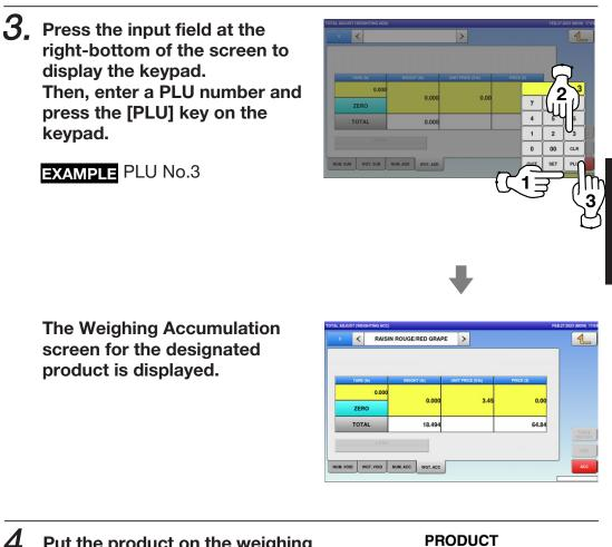
**4.** Put the product on the weighing platter and press the [ACC] button.
