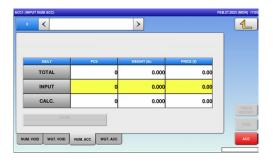
2. Press the input field at the right-bottom of the screen to display the keypad. Then, enter a PLU number and press the [PLU] key on the keypad.
