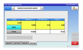
**4**, Put the product on the weighing platter and press the [ADD] button.
