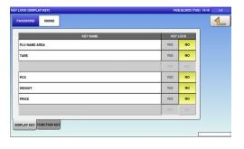
2. Press the "FUNCTION KEY" tab to display the "Key Lock (Function Key)" screen. To turn pages, press [▼] or [▲].
