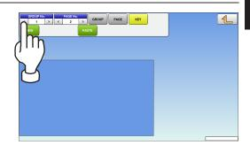
**4.** To create or delete the group or the page, press the [GROUP] or [PAGE] button, and then press a desired function button as shown below.
