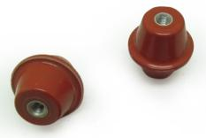
Power surges such as those caused by welding or electrical shorts frequently damage load cells and indicators. To prevent such damage, these isolators electrically separate the mechanical assembly from its tension-type load cell.
