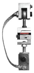
Module with RL20000ST S-beam load cell
