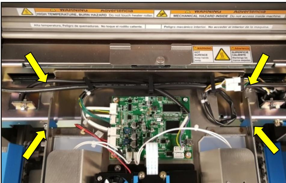
Figure 7. Camera Housing Mounting Bolts
