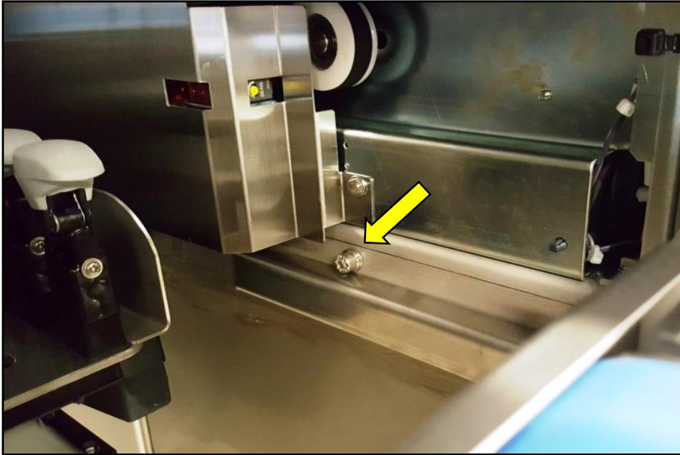
Figure 2. Socket Head Stopper Bolt – Right Side
