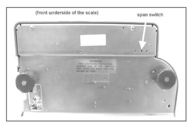
Figure 4-1. Location of Span Switch
