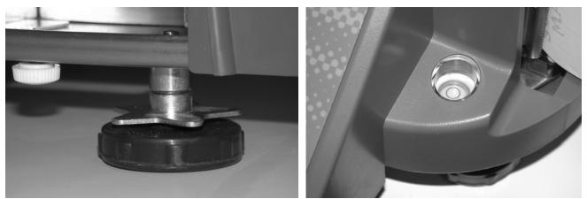
Figure 2-2. Leveling Feet and Bubble
