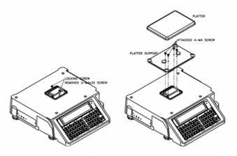
Figure 2-1. Unlocking the Scale and Installing the Platter Support
