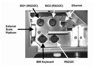
Figure 12-1. DC-200/300 Interface Ports
