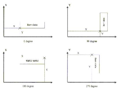
Figure 7-39. Starting Positions for Print Angles
