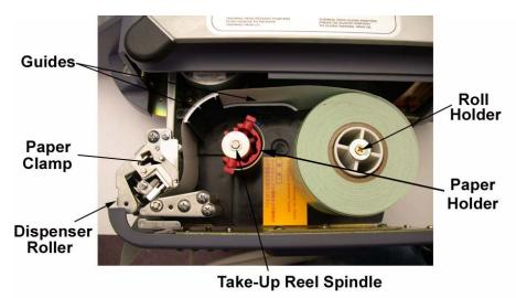
Figure 7-20. Loading DC-300 Printer
