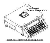
Remove the bag protecting the scale and the dessicant bag. and the protective film covering the front panel. The rest of the unpacking/unlocking procedure depends upon the capacity of the scale.
