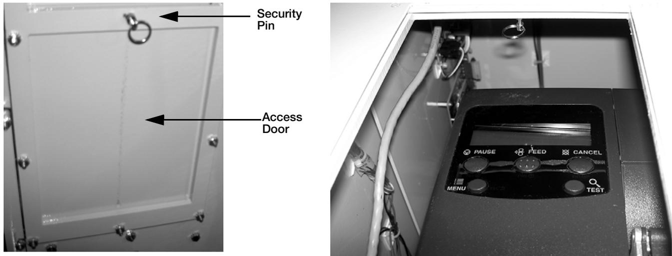
Figure 2-1. In-kiosk security pin release for printer access door (left); Printer revealed with access door raised (right)
