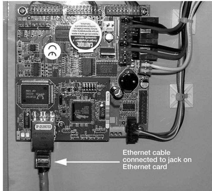
Figure 2-2. Ethernet Cable Connection
