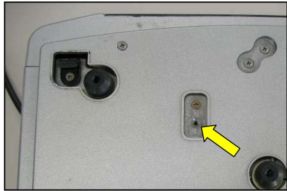
Figure 9.2. Calibration Access
