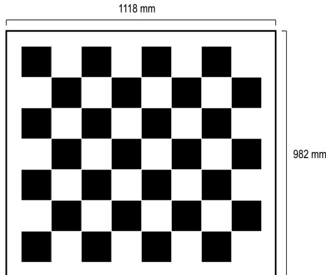
Figure 5-2. Calibration Object
