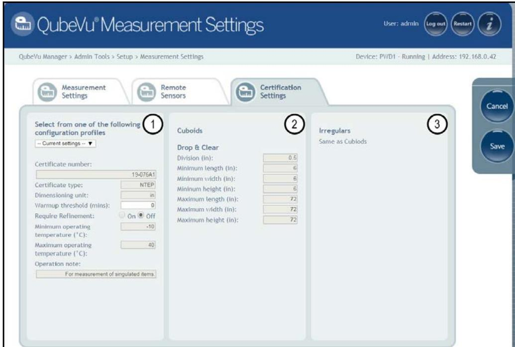
Figure 4-5. Measurement Settings Tab
