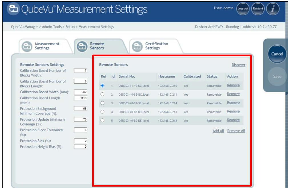
Figure 4-4. Remote Sensors: Discovery Settings
