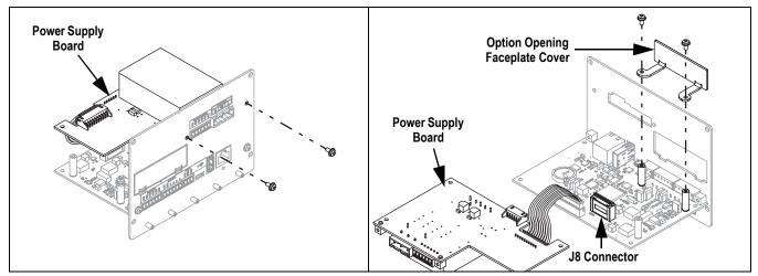
Figure 3. Power Supply Board and Faceplate Cover Removal
