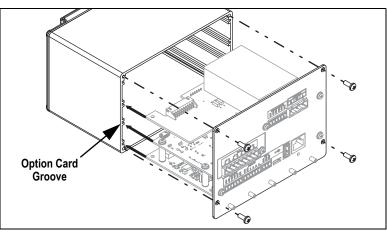
Figure 5. Backplate with Boards Reassembly
