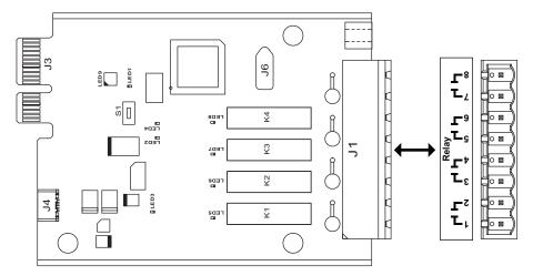
Figure 7. Relay Option Card Board
