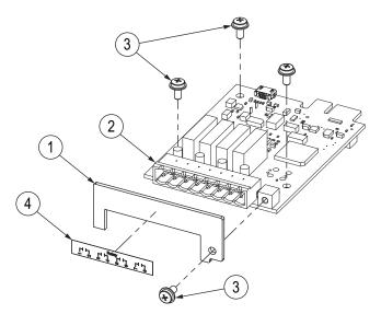
Figure 1. Relay Option Card Parts Breakdown
