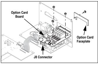
Figure 4. Option Card Board and Faceplate Installation
