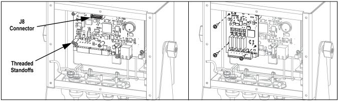
Figure 6. Option Card Board Installation
