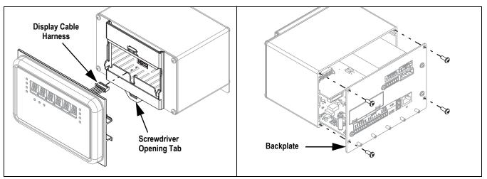
Figure 2. Front Panel and Backplate Removal
