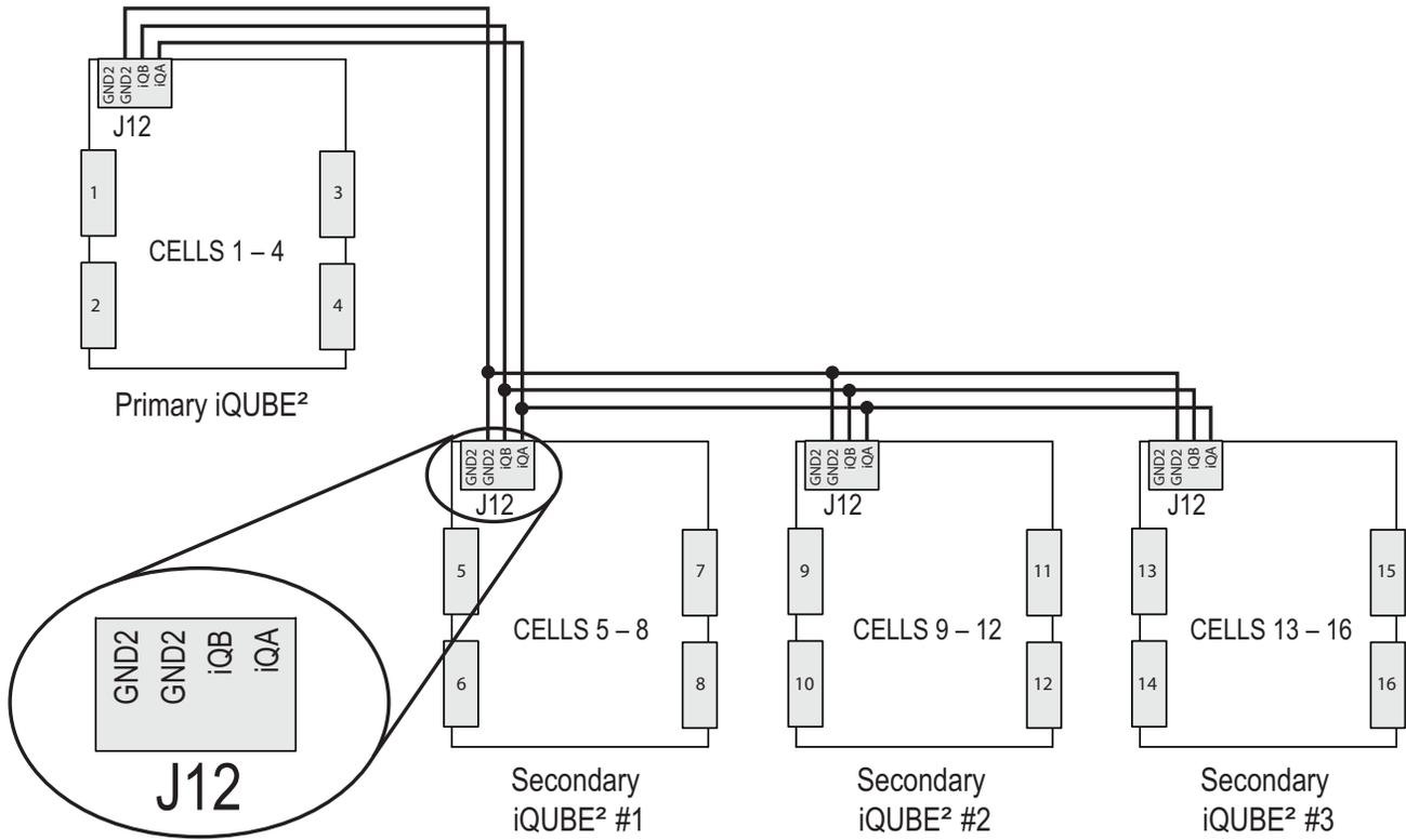
Figure 8. Primary-to-Secondary Communications Wiring
