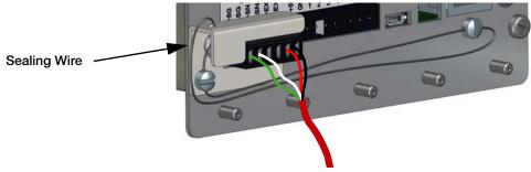
Figure 2-22. Install Sealing Wire
