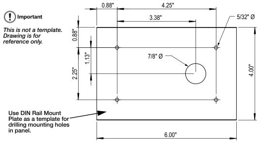
Figure 2-2. Pattern for Cutting Holes
