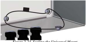
Figure 2-23. Sealing the Universal Mount
