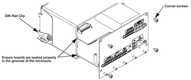
Figure 2-12. Boards Installed in Controller Assembly Enclosure
