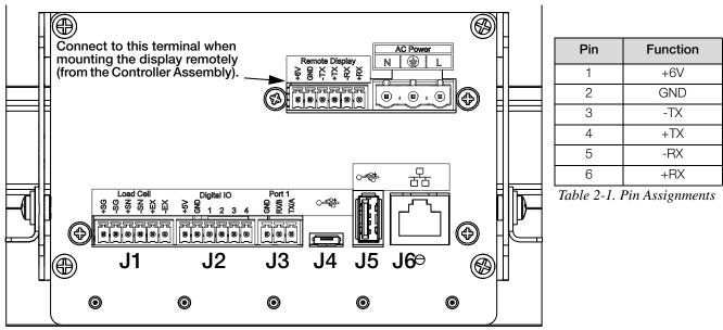
Figure 2-5. Mount Controller Assembly Remotely
