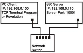
Figure 9-2. Connection from PC to 880 Ethernet Through a Network Switch or Router
