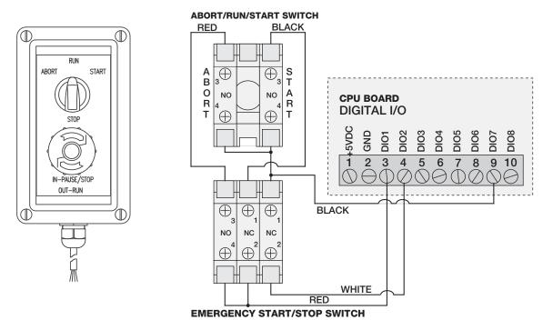
Figure 8-1. Batching Switch and Wiring Diagram Example
