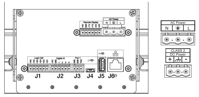
Figure 2-17. Power Connection Location
