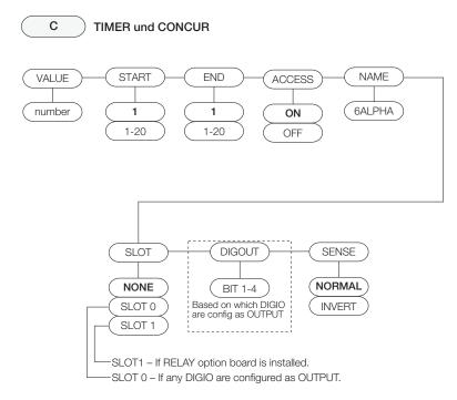
Figure 3-18. Setpoint Menu Structure – Layout C
