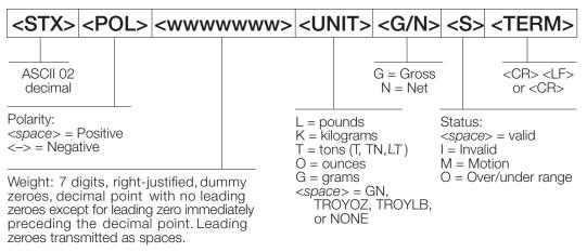
Figure 10-1. Stream Serial Data Format – RS-232 and RS-422
