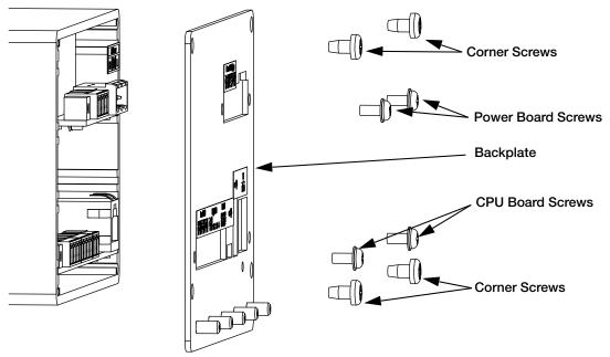
Figure 2-8. Remove Controller Assembly Backplate
