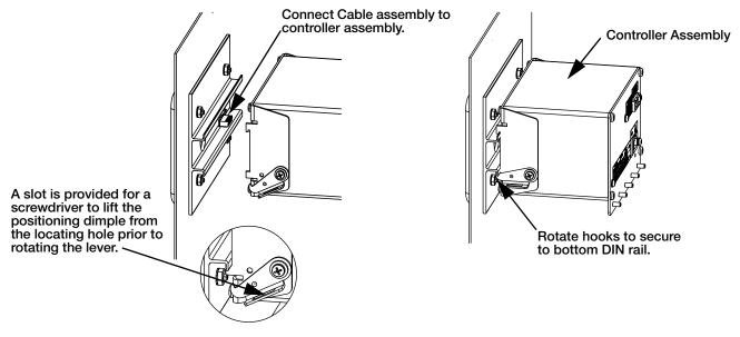
Figure 2-4. Install Controller Assembly
