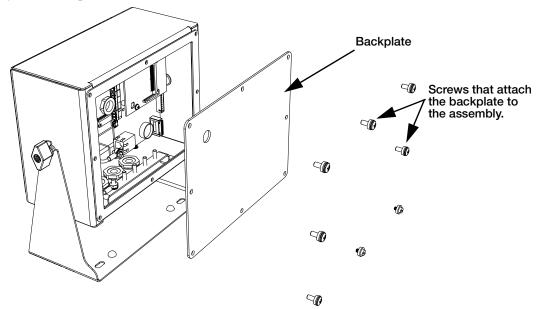
Figure 2-14. Remove Universal Mount Backplate
