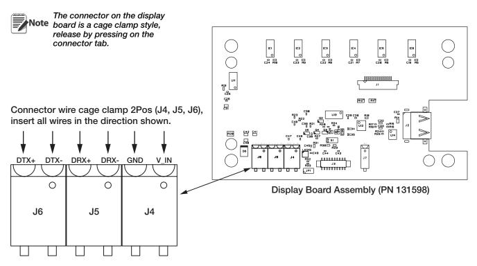
Figure 2-6. Wire connection to Display Board
