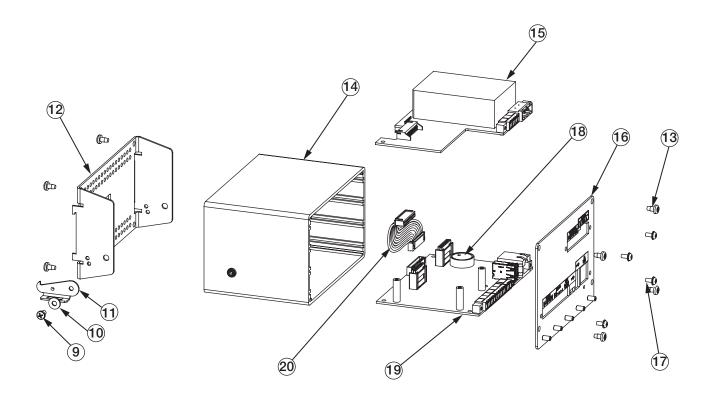
Figure 2-24. 880 Indicator Parts Illustration
