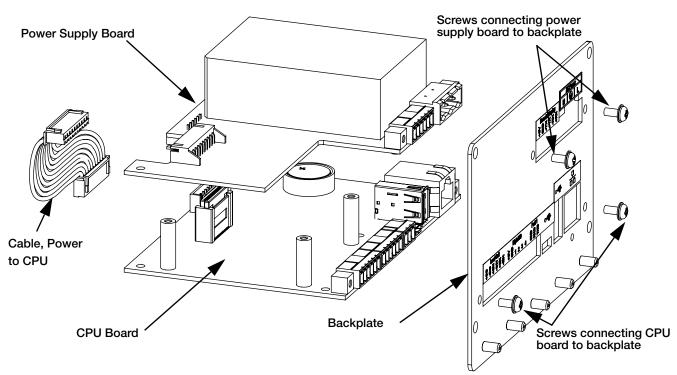
Figure 2-11. Boards Removed from Enclosure
