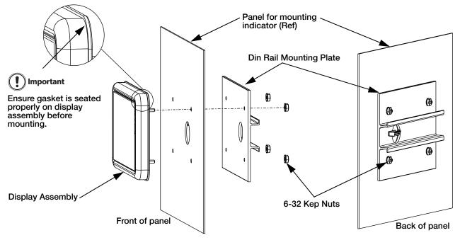
Figure 2-3. Mounting Display Assembly
