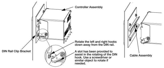
Figure 2-7. Remove Controller Assembly
