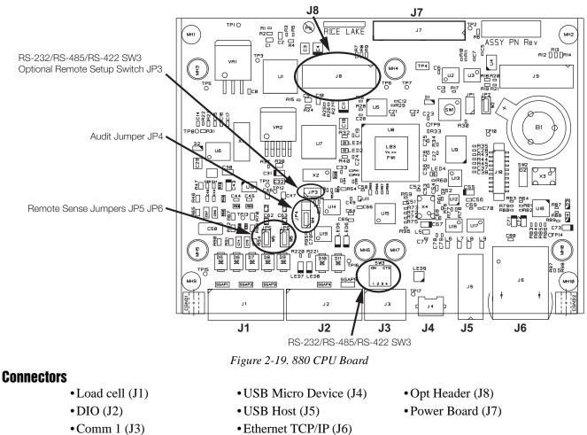
The COMM 1 port supports RS-232 or two-wire RS-485/RS-422 communications; selectable with switch SW3. The port is configured using the COM menu under Ports. See Section 3.0.
