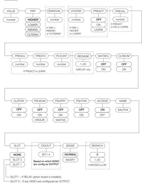
Figure 3-16. Setpoint Menu Structure – Layout A
