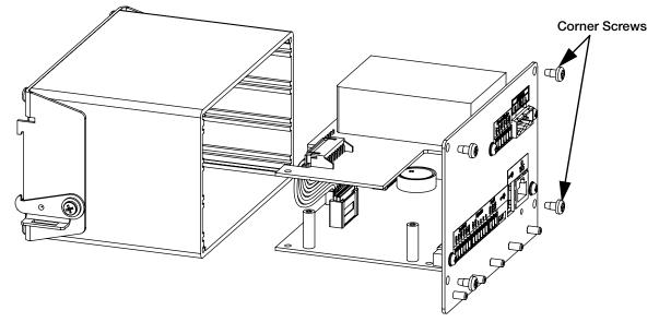
Figure 2-10. Remove Backplate With Boards
