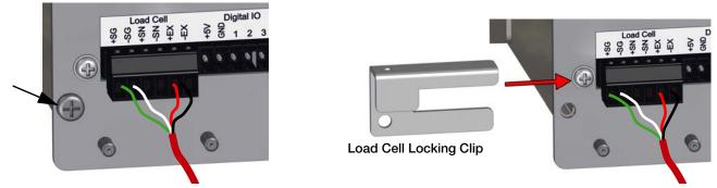
Figure 2-21. Remove Existing Screws
