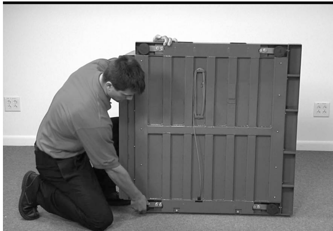
Figure 2-3. Backing out the Scale Feet
