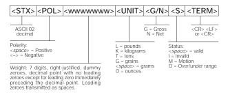
Figure 10-1. Continuous Output Serial Data Format
