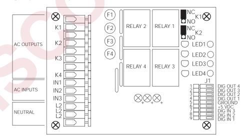
Figure 9-15. IQ plus 800 4-Channel Relay Board, PN 36080
