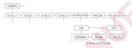
Figure 9-2. Peak Hold Submenu
