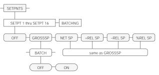
Figure 8-3. Setpoint BATCH Parameter
