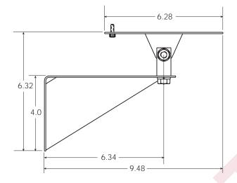
Figure 2-10. IQ plus 810 Wall Mount (Side View)
