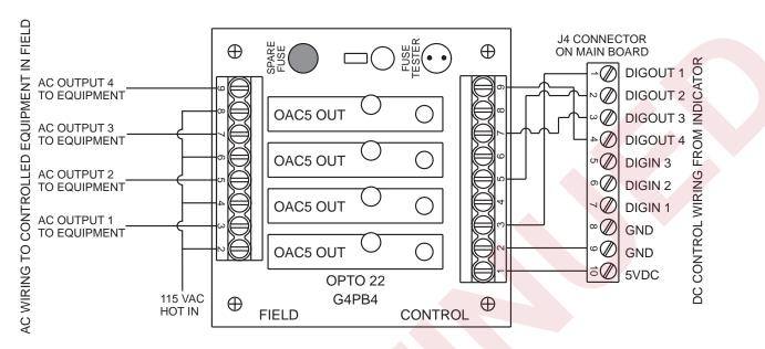
Figure 9-19. Relay Wiring for 4 AC Outputs
