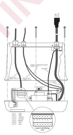
Figure 2-2. IQ plus 810 Wiring, Top View
