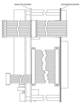
Figure 9-8. Installed Expansion Board, Side View
