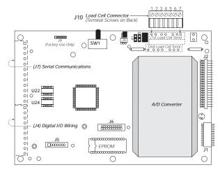
Figure 2-5. CPU Board, Component Side
