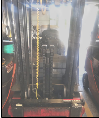
Figure 2. Inadequately Secured Coiled Cable
