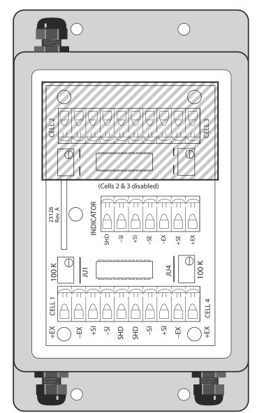
Figure 3-1. DeckHand Junction Box Cutaway
