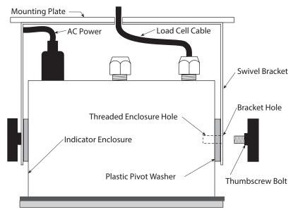
Figure 2-2. Top View of Indicator and Bracket
