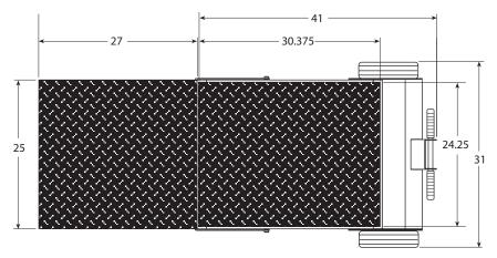
Figure 3-4. Scale and Ramp Dimensions (Inches)
