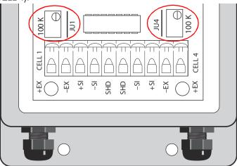
Figure 3-2. Cell 1 and Cell 4 Potentiometers
