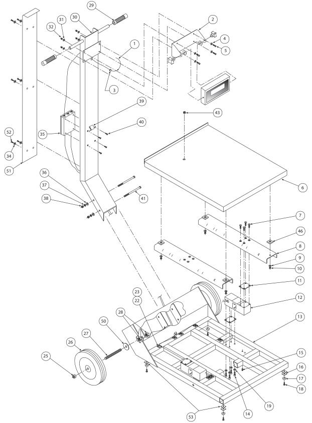
Figure 4-1. Replacement Parts Illustration
