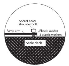
Figure 3-5. Ramp Pivot Bolt
