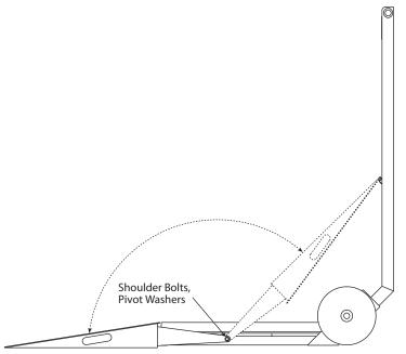
Figure 2-1. Pivoting Ramp
