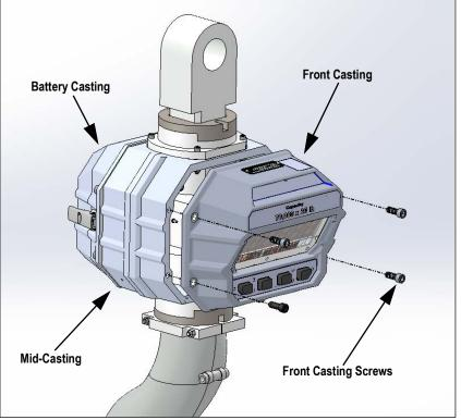
Figure 2. Front Casting Removal
