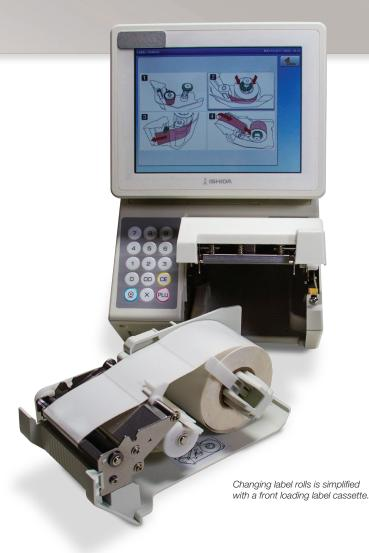
The WIL-Acro II compact label printer features ultra-fast printing speeds and a front-loading label cassette. The color touchscreen streamlines operation and its compact size is ideal for applications with limited space. such as floral counters and bakeries.
