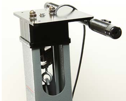
Figure 4-4. Run Load Cell Cable Through Base Plate and Tighten Base Plate to Pillar
