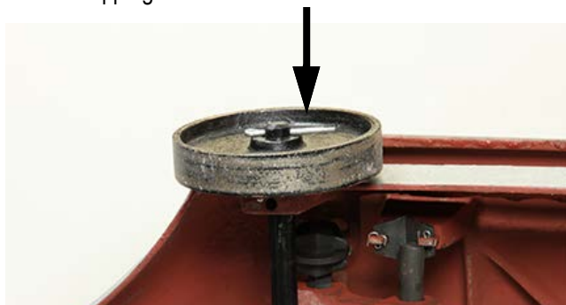
Figure 2-4. Run Cotter Pins Through Wheel Axle Holes to Prevent Slipping
