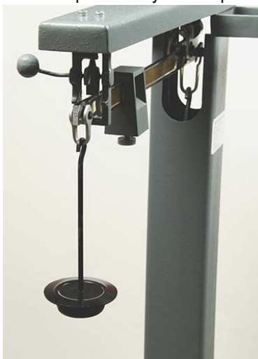
Figure 2-17. Hanging Counterpoise Assembly
