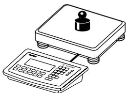
▶ Place a sample with the target weight (in this example, 1250 g) on the platform.
