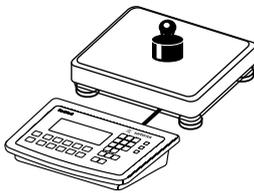
▶ Place a sample with the target weight (in this example, 1250 g) on the platform.
