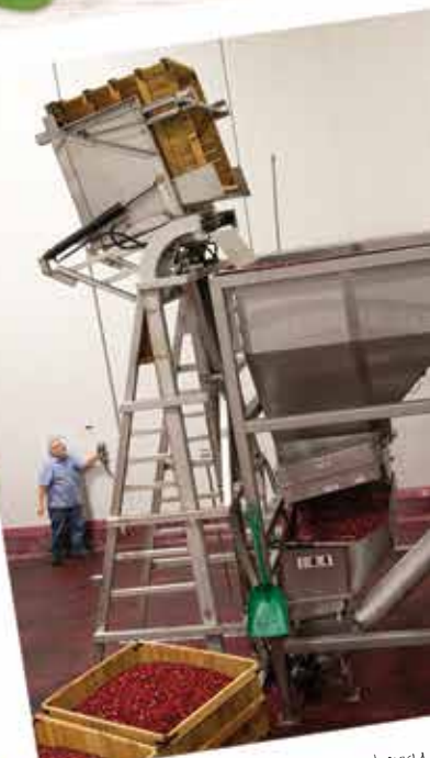
The hopper breaks up berry clusters before the metal detection.
