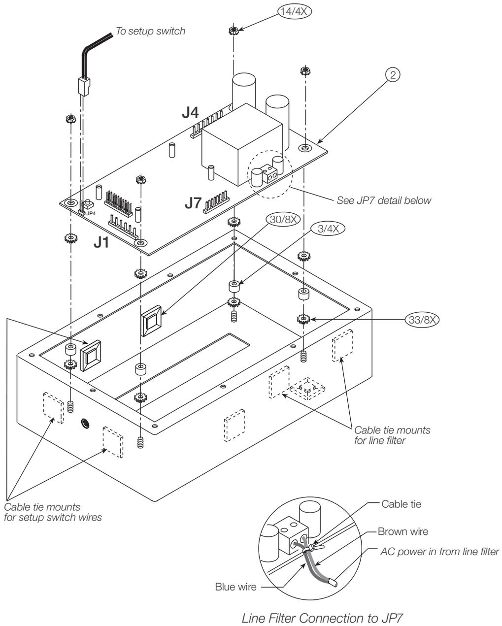
Figure 2-6. IQ plus 355 Enclosure and CPU Board
