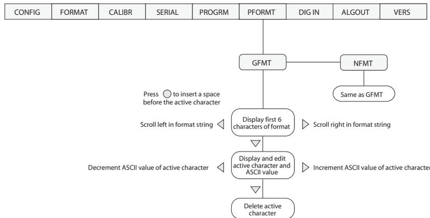
Figure 5-1. PFORMT Menu, Showing Alphanumeric Character Entry Procedure
