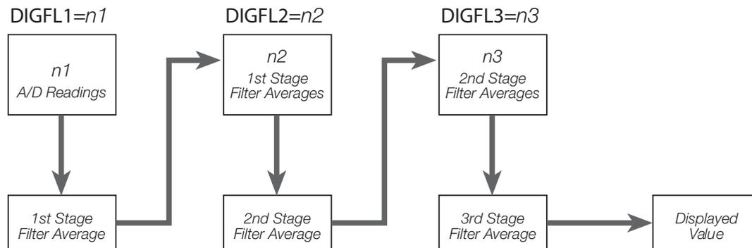
Figure 7-4. Flow Diagram for IQ plus 355 Digital Filters
