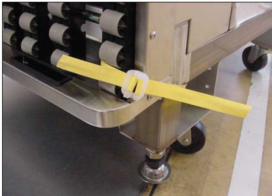
Figure 7. Securing the Exit Conveyor
