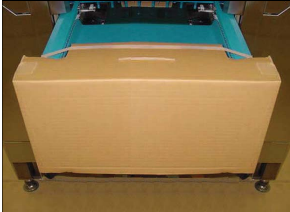
Figure 8. Infeed Covered to Prevent Damage
