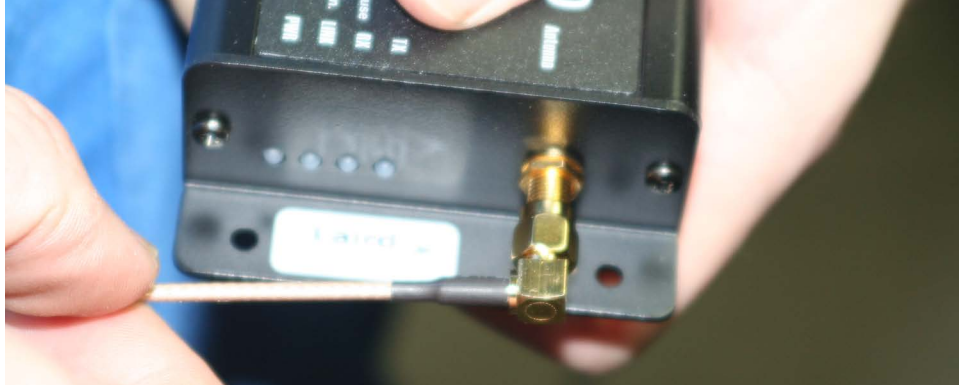
Figure 7. Attach Cable Extension Antenna to ConnexLink Wireless Radio
