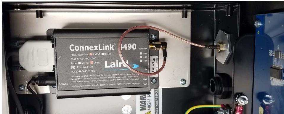
Figure 8. Mount ConnexLink Radio to Bracket
