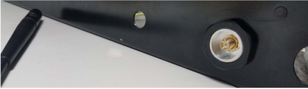
Figure 4. Thread Antenna Extension Cable Through
