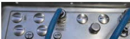
Menu Access Switch/Calibration Switch Cover
