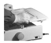
**3** Pull up on the lock levers and open the tractor covers. Then, move the right tractor to fit the width of the paper.
