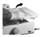
5 Install the paper separator. Install the pull-up roller assembly. Close the access cover.
