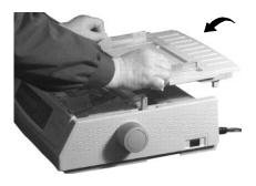
8 Install the pull-up roller assembly. Close the access cover.
