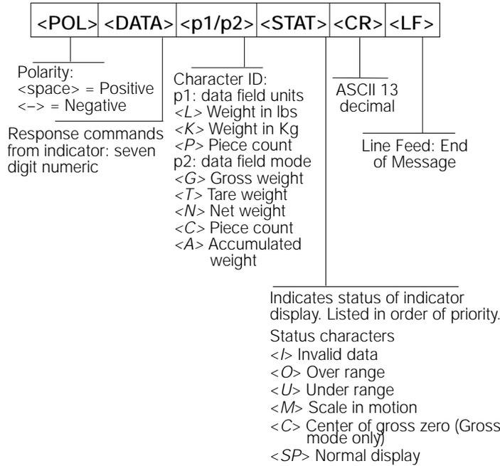
Figure 8-2. Continuous Default Output Serial Data Format
