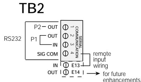
Figure 2-8. Alternate Serial I/O wiring
