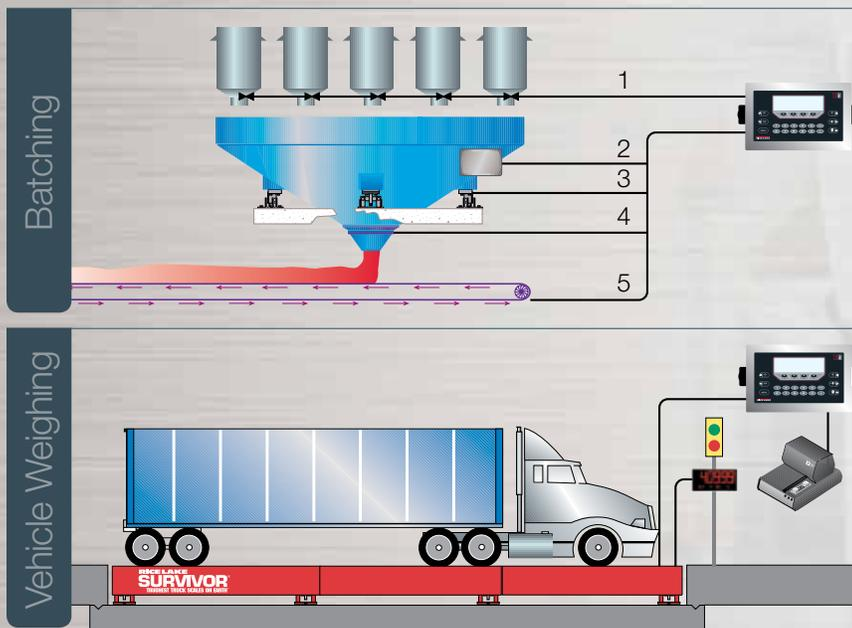
This sequence is one example of a simple process programmed using the 720i's standard batch engine. (1) At the touch of a button, gates release product into a large hopper. (2) The product is then measured using weight data collected from load cells. (3) Next, the 720i signals a motor to mix the hopper contents for a given length of time. (4) Lastly, another gate is engaged to discharge a certain amount of product based on weight, (5) while a conveyor system is simultaneously activated.
