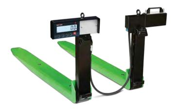
The RL-MFW is designed for light duty indoor use to accurately weigh pallets throughout warehouse environments with Legal for Trade approved accuracy. Install on any forklift carriage class type Fem IIA or IIIA using a DIN 15173 FEM holder plate. Provides legal weight without derating lift truck capacity.
