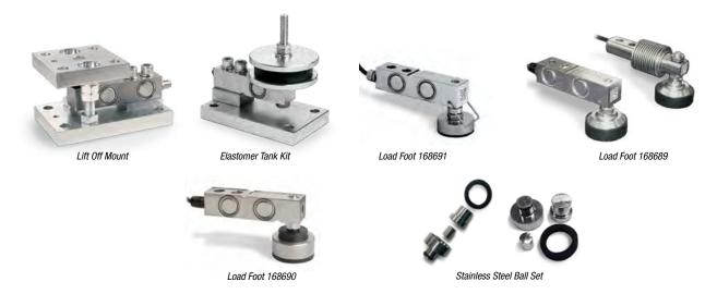
Complete mounting solutions for the RL35 single-end beam load cell. Lift-off mount provides protection for the RL35 load cell. Mounting solutions available in alloy or stainless steel. Base plate is available to fill application needs for plate only. Lift-off silent block works in conjunction with base plate to provide correct protection. Ball set provides correct oscillation for mounting applications.
