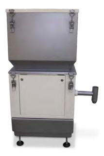
With Loss-In-Weight, the weight reduction per time interval is measured and integrated to a flow. A regulation can then be added to create a closed regulation loop by dosing. Product could be conveyed by a screw conveyor, vibrating conveyor, belt conveyor or others. The scale by itself, or the complete system with dosing conveyor can be purchased.
