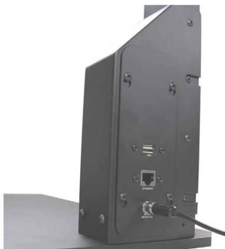
Figure 3-21. AC Power Connection
