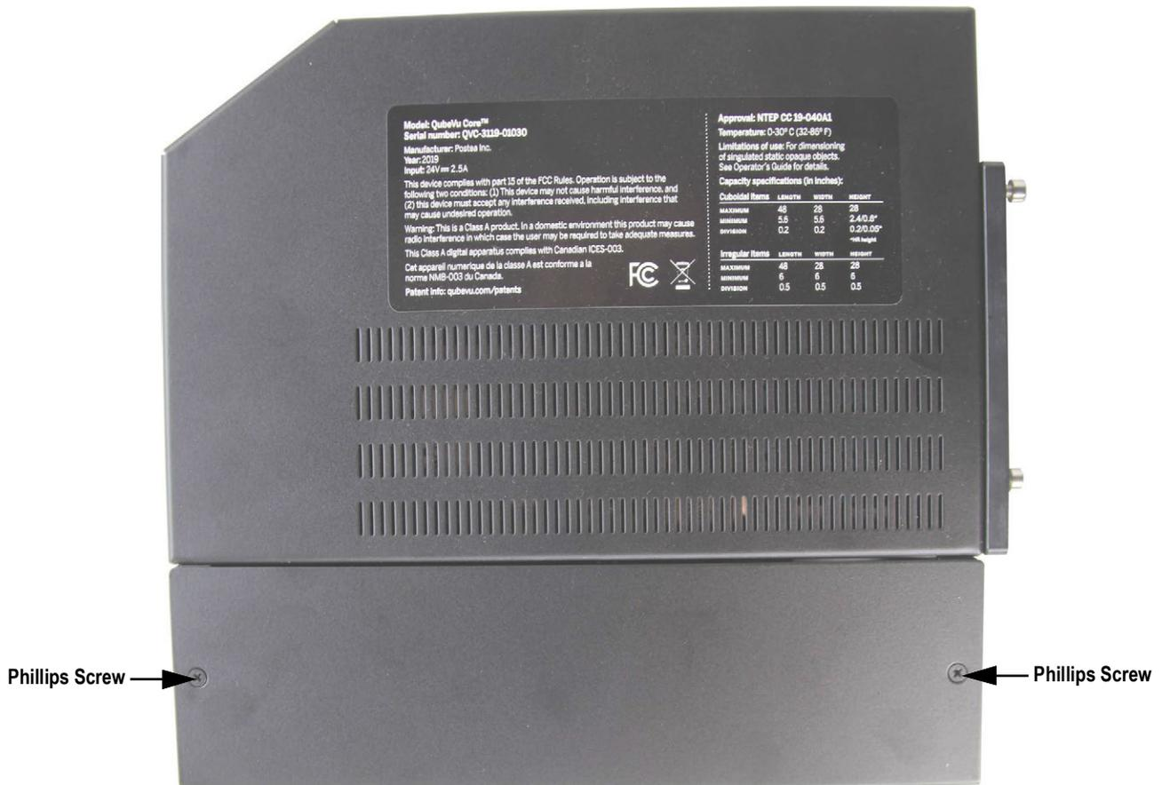
Figure 3-18. Scanning Head with Rear Cover Secured
