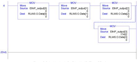
Figure 3-5. Ladder Logic for EtherNet/IP (Two of Two)
