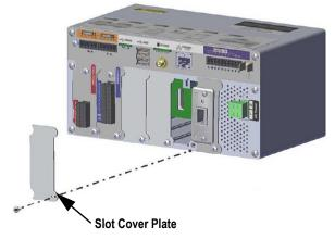
Figure 2-2. Existing Cover Plate Removal
