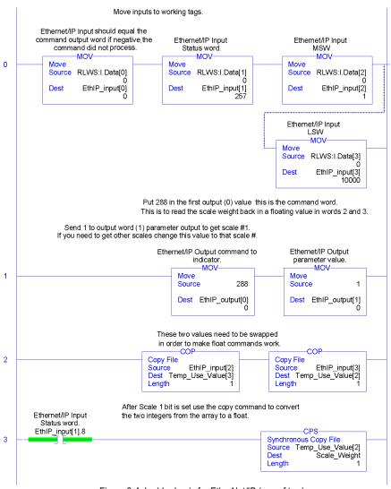
Figure 3-4. Ladder Logic for EtherNet/IP (one of two)
