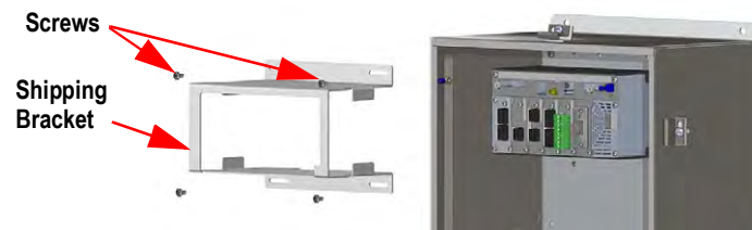
Figure 2-9. Remove Shipping Bracket
