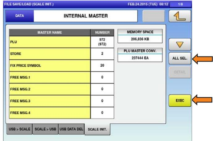
Figure 4-3. USB Memory Stick Input to Scale Memory
