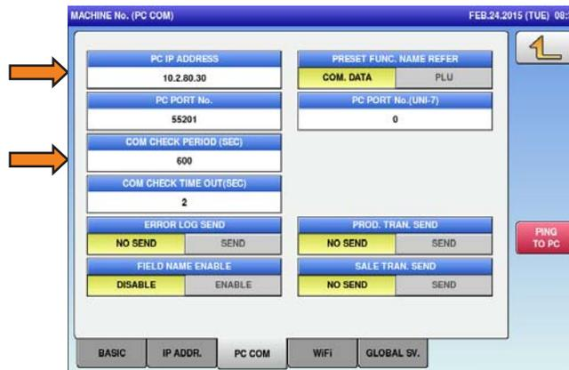
Figure 3-2. IP Address and Com Check Period
